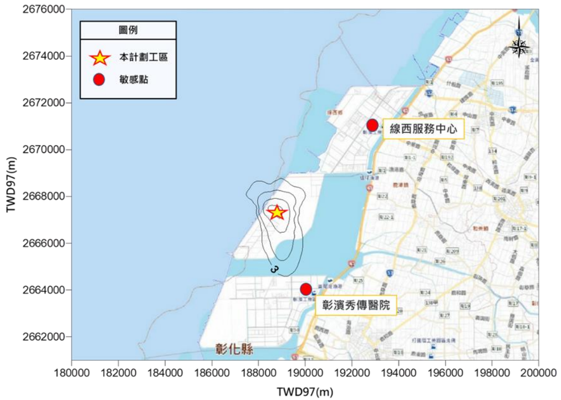
Figure 6.1.2-1 Simulation of Max Increase in Value of 24 Hours for TSP during Onshore Construction
