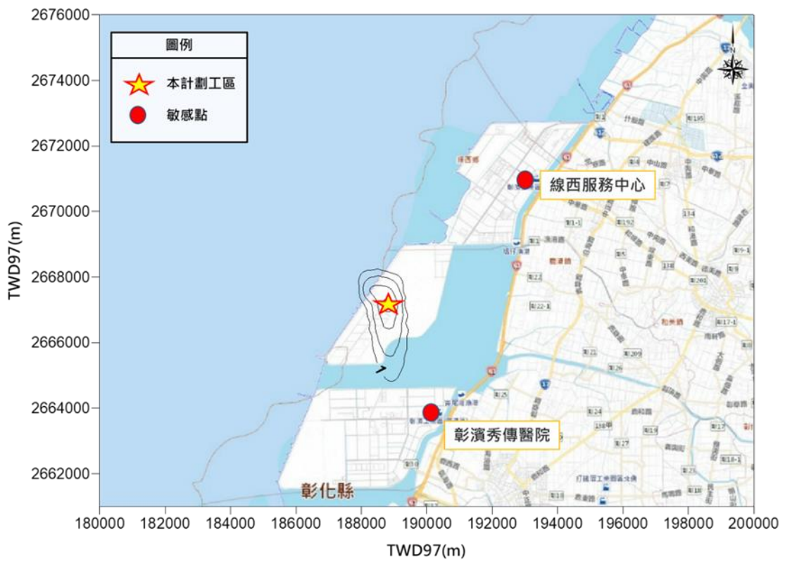
Figure 6.1.2-2 Simulation of Increase in Annual Average Value for TSP during Onshore Construction
