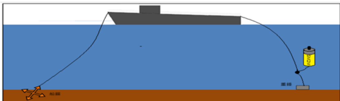
Figure 6.2.4-3 Schematic Diagram of Underwater Noise Measuring Equipment Deployment
