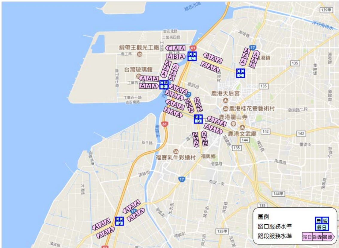
Figure 7.5-2 Schematic diagram of the surrounding road service level during the construction phase (2)
