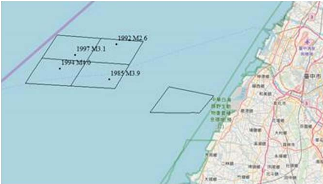
Fig 7.7.2-2 Seismic focus that occurred in the wind field of the project
