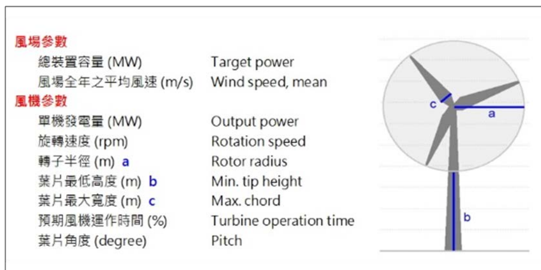
Figure 7.2.4-3 Simulation Diagram of Parameter of Wind Turbine Needed In Different Band Model
