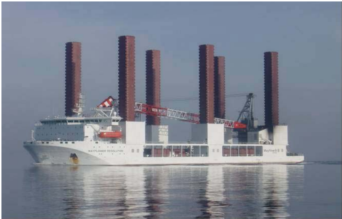
Jackup barge "Mayflower Resolution", which installs the wind turbine at Barrow Offshore Windfarm.
