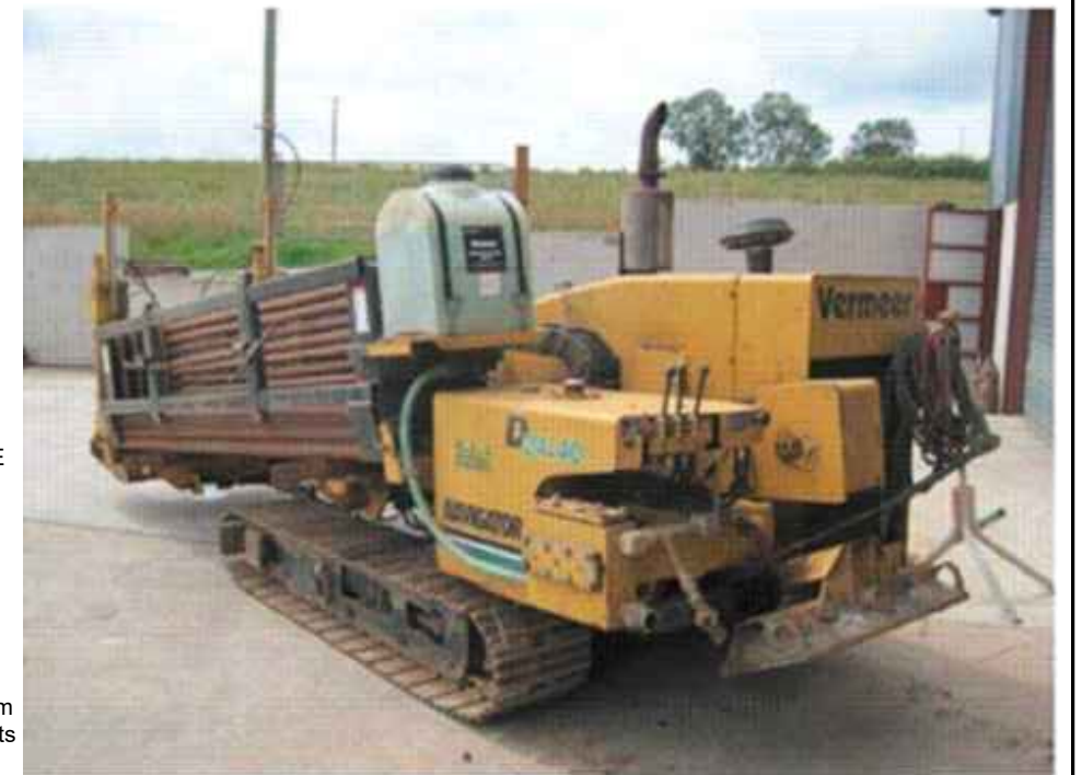
Directional Drilling Rig
