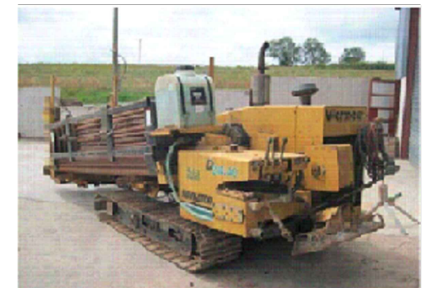
DIRECTIONAL DRILLING RIG
