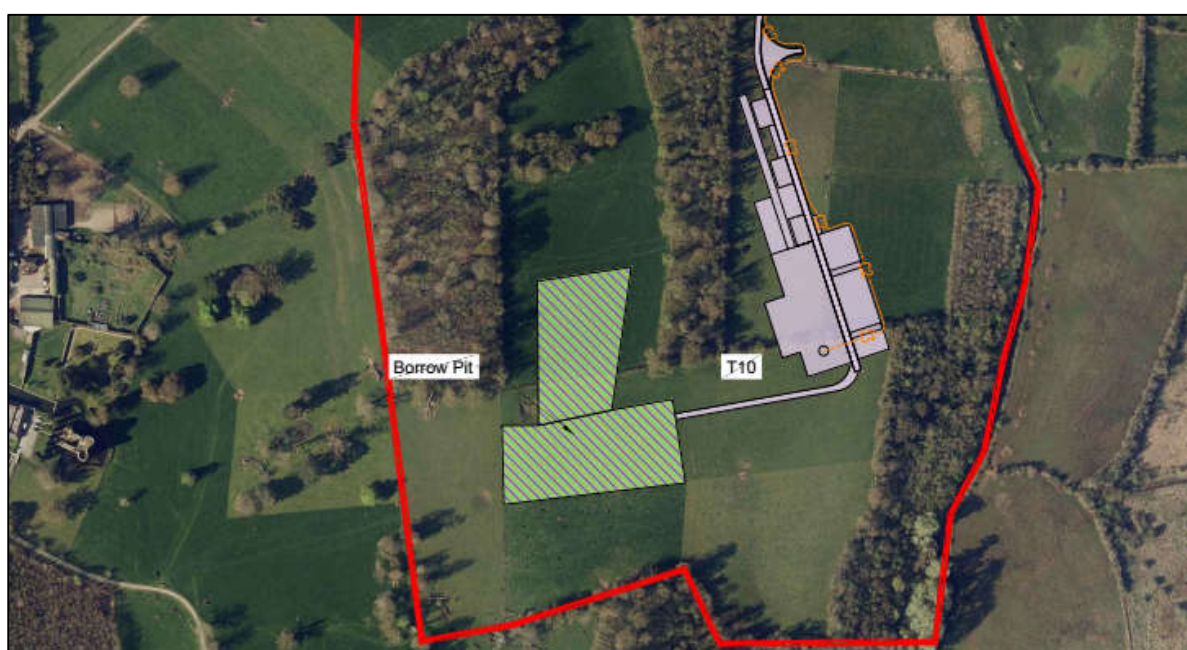
Figure 8-14: Green hatched area showing Borrow Pit/Material Storage Location west of Turbine 10 which will also act as a deposition area.
