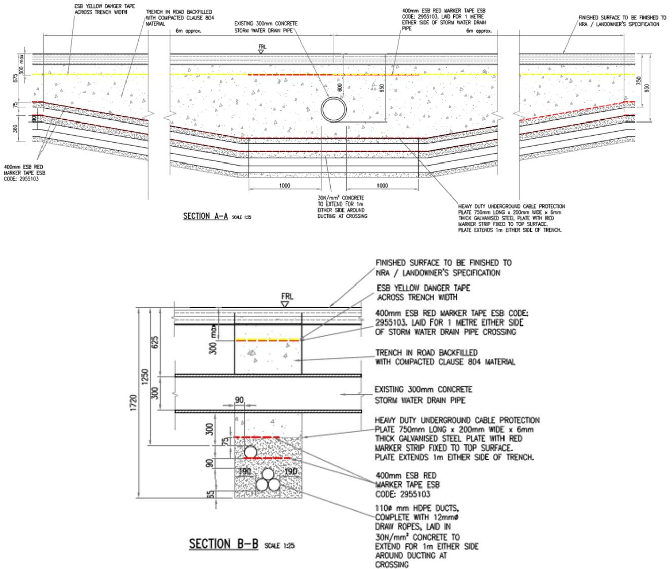
**Plate 3-3: Piped Culvert Crossings – Ducting under Culvert Crossing Details**
