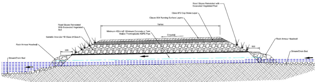
**Plate 3-5: Piped Culvert Crossing Long Section**
