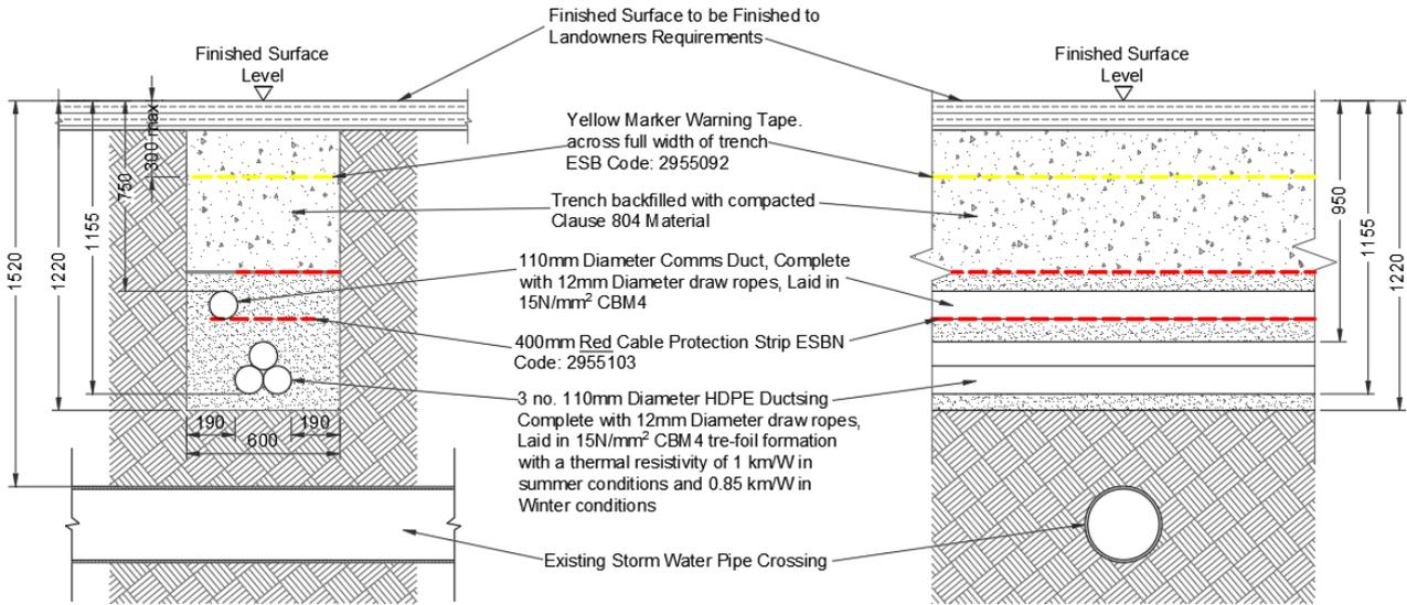
**Plate 3-2: Piped Culvert Crossing – Ducting Over Culvert Crossing Details**
