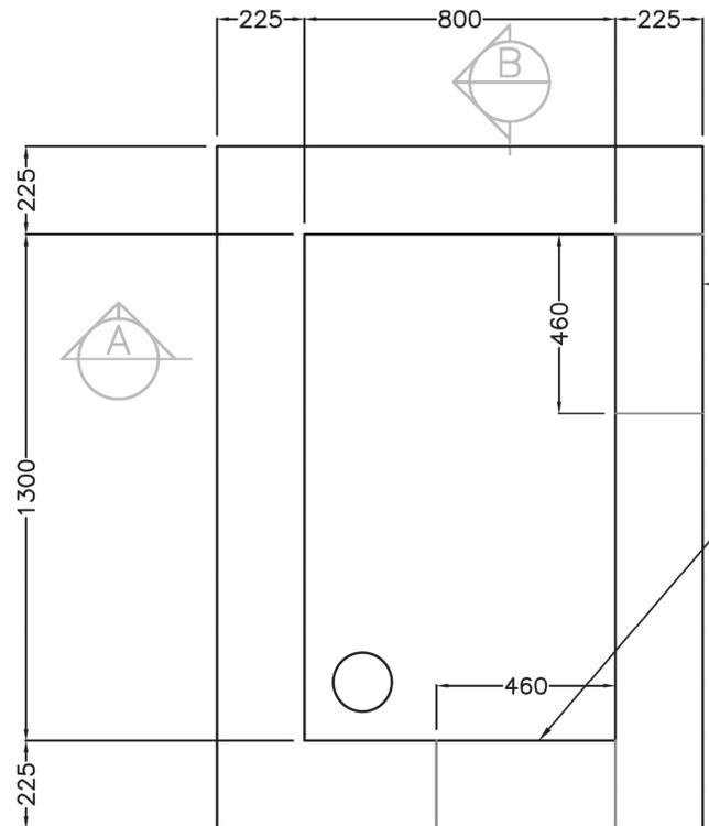
WALL OPENING 460x325 MAX. ACTUAL SIZE TO BE FORMED TO SUIT DUCT ENTRIES. VOIDS TO BE SEALED AND SURFACES MADE GOOD WITH CLASS 1 MORTAR.
