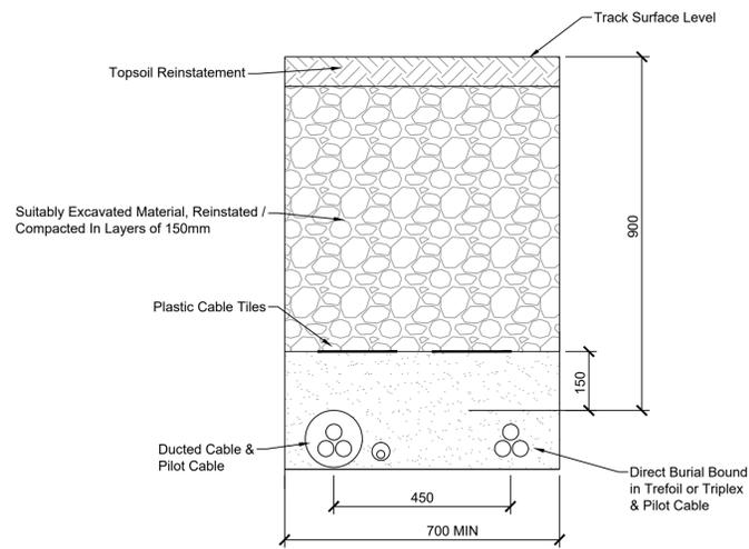
**TRENCH CROSS SECTION - PILOT CABLES**
