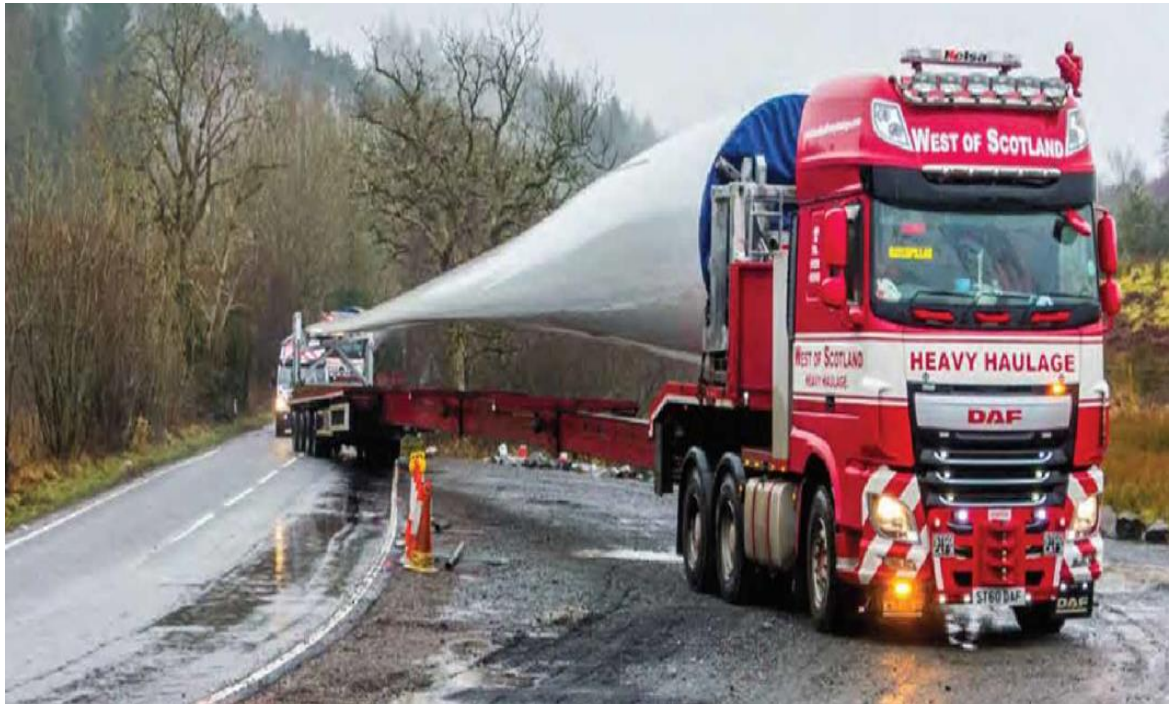
Image 4: Typical Abnormal Load Vehicle Transporting Turbine Blade
