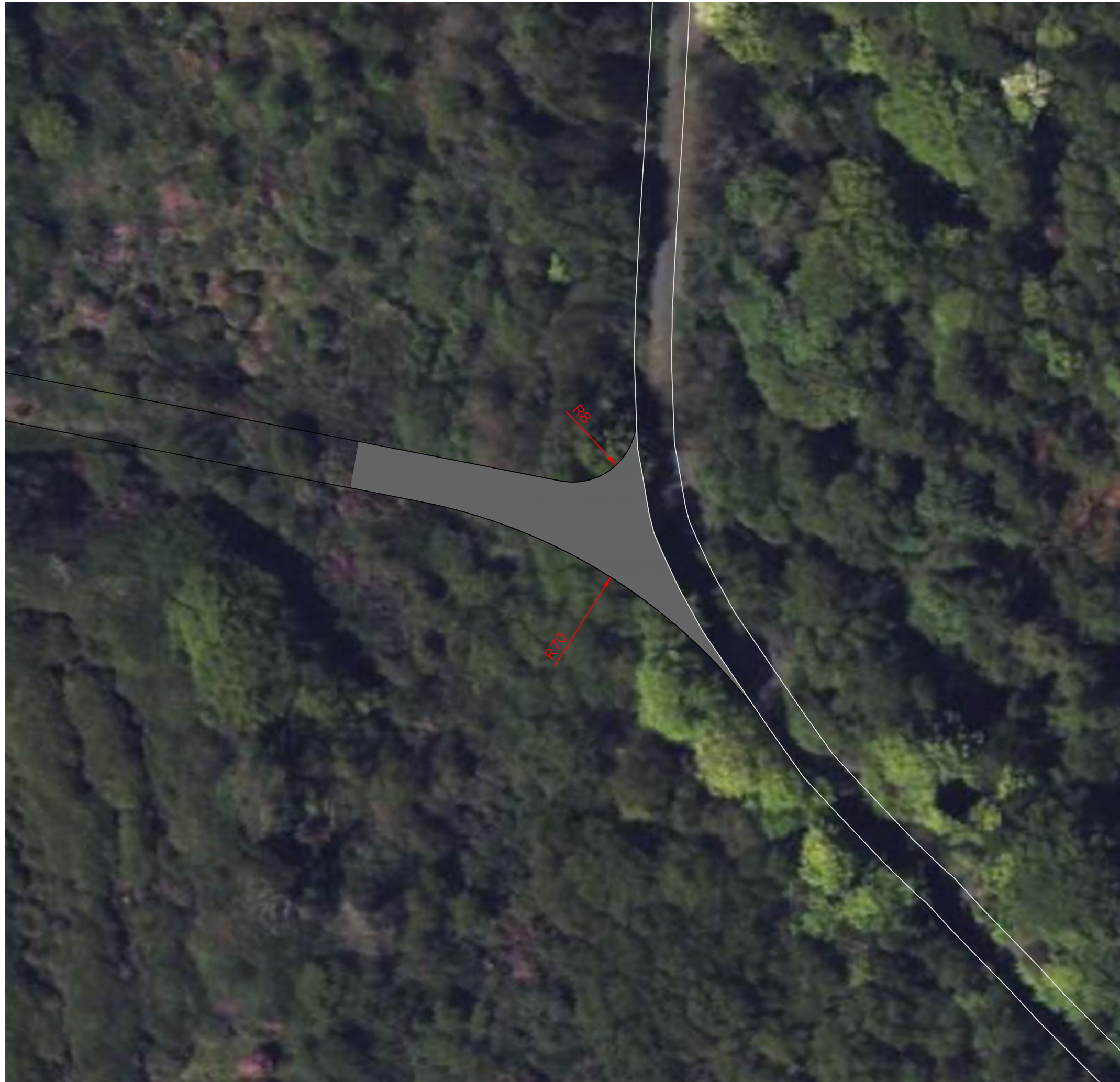
Figure 4.8: Indicative New Site Junction
