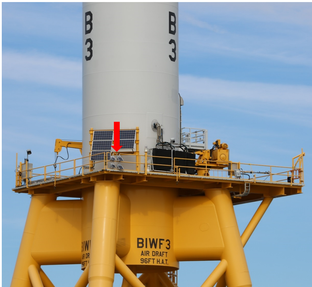
Figure 2. Two acoustic bat detectors (1 primary and 1 backup) and two acoustic bird recorders (1 primary and 1 backup), indicated by red arrow, deployed on the south-facing railing of the platform on Turbine 3 at BIWF.
