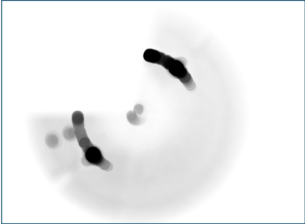
Figure 4-1 Radar mask. Images shows the mean level of masking during the month of May 2020. The intensity of black color reflects the frequency of masking during this month.
